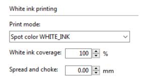
You can generate White ink either by mapping a spot color (if one exists in the input job) or by using one of the available options: Bounding Box (Flood), Inked Image or Inked Image Inverse. Details of creating white calibration is available in the Advanced Calibration Guide.
